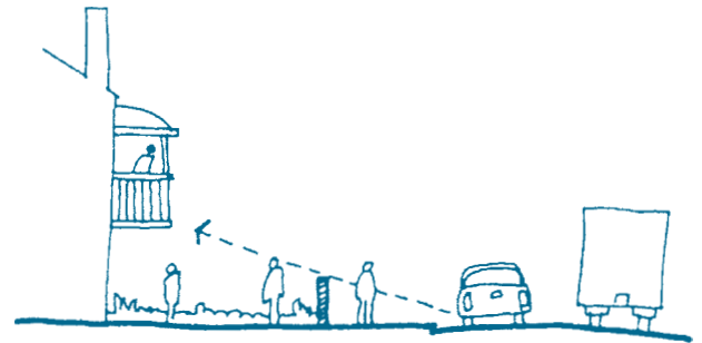
Figure 5: A low front fence will block some noise and allow interaction and surveillance.
