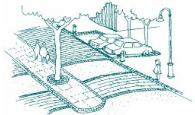
Figure 1: Pavement treatments and materials can contribute to an attractive streetscape and enhance traffic calming.
